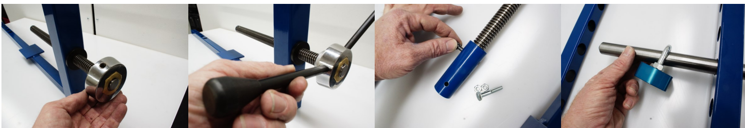
Thread hand wheel on to threaded rod. Screw in handles. Attach coupler to threaded rod with supplied screws. Slide extractor rod through frame arm holes and through extractor U bolt.
