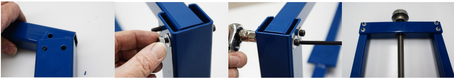
Slide right and left frame arms into top extractor frame. Using provided nuts, bolts, and washers, screw both arms into place on top frame. Ensure washers are on both sides of frame. Using allen wrench and open wrench to tighten nuts. Drop threaded rod into bushing.
